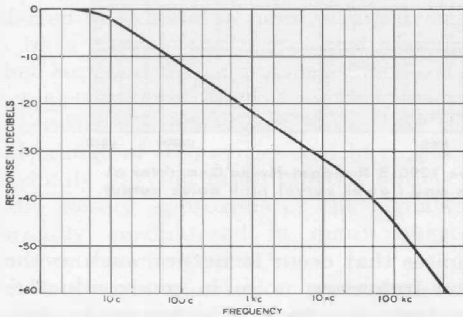
Attenuation-frequency characteristic of the Pink-Noise Filter.
